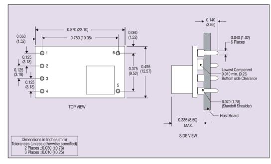
Figure 6 - Plated Through-Hole Mechanical Drawing
