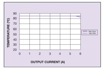
Figure 3 - Safe Operating Area for PTH12050L Vin = 12 V, Output Voltage  $\leq$  1.8 V (See Note A)
